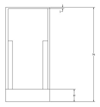
WIDTH D.D. 35 1/2" DEPTH D.D. 36 1/4" HEIGHT D.D. 76"
