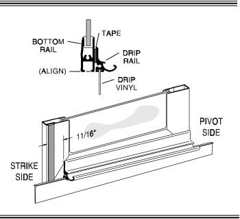
Adjust the drip vinyl [W] by sliding it left or right until it just touches the curb. Trim the vinyl (flush with the pivot end and notch 1/4" longer than the drip rail as shown on the strike end). Secure it with one #6 x 3/8" truss head screw [E] in the pivot end of the drip rail.
