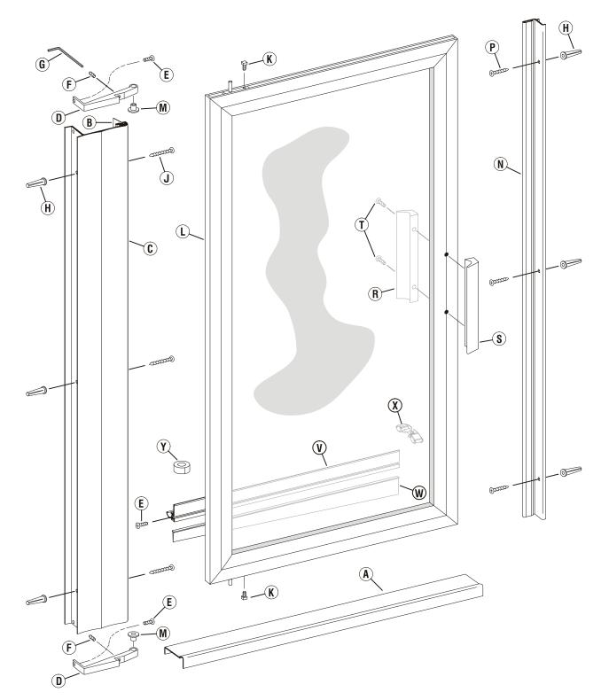
The 738 Pivot Shower Door is completely reversible and may be installed pivot-right or pivot-left. Using the diagram, determine the correct position for your installation. For maximum waterproofing, the pivot jamb should always be opposite the shower head. These instructions depict a pivot-left installation.
