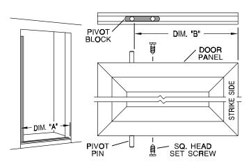
Insert a nylon pivot bushing [**M**] into the bottom pivot bracket [**D**]. Slip the second pivot bushing over the top pivot pin on the door panel. Position the door by inserting the bottom pivot pin into the bottom pivot bracket. Hold the door vertical and slide the top pivot bracket into the pivot jamb [**C**] and over the top pivot pin and pivot bushing. Secure the top pivot bracket with a #6 x 3/8" truss head screw [**E**] and a #8-32 x 1/8" Allen set screw [**F**].
